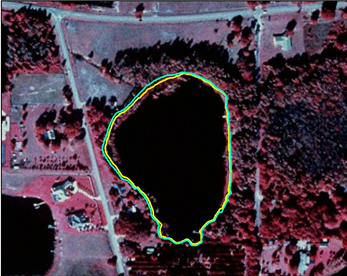
Figure 4. Approximate location of the proposed Minimum Lake Level (yellow) and proposed High Minimum Lake Level (blue) for Lake Jackson in Hillsborough County, Florida. Elevations listed are in feet above the National Geodetic Vertical Datum of 1929.
